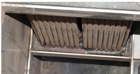
Figure 4: Air side fouling after 18 months in an area with heavy industry
