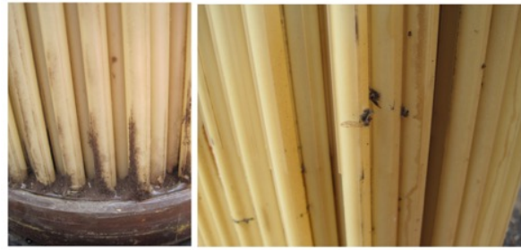
Figure 5: Air side fouling after 6 months in a rural environment
